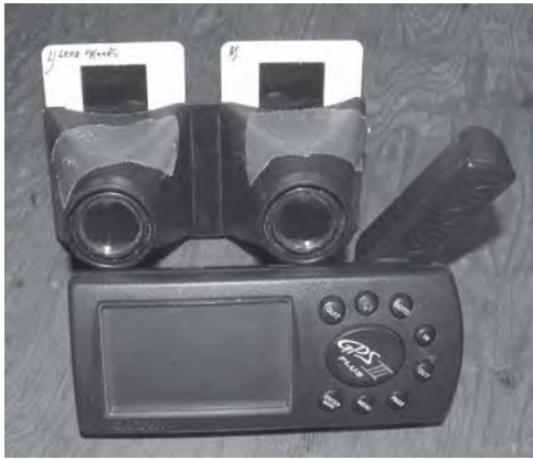
Fig 1.4 GPS unit and stereo slide viewer. The 1984 true color aerials (Fig 1.1b) were copied as 35 mm slides and inserted into this viewer, providing a 3D terrain image useful in field navigation.
