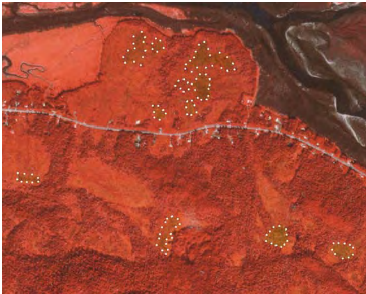
Fig 1.2 1979 NASA color infrared aerial, 1:63,360. On this vintage photography (but less so on subsequent CIRs) the wettest portions of sphagnum bogs with greatest density of small ponds can be identified from greenish tints. These patches are outlined here with white dots. Fens are distinguishable from bogs by their paler peach color.
